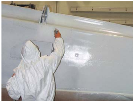
Figure 3. Zero-VOC Topcoat Application to Outer Wing Panel of C-2 (left) and F/A-18D at NADEP NORIS (right).
