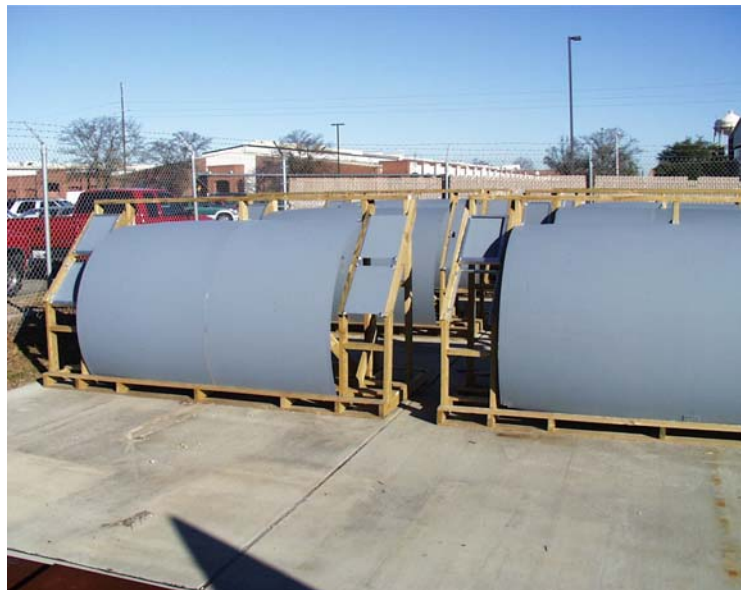
Figure 2. Condemned C-141 Aft Cowlings Exposed at WR-ALC for 14 Months.
