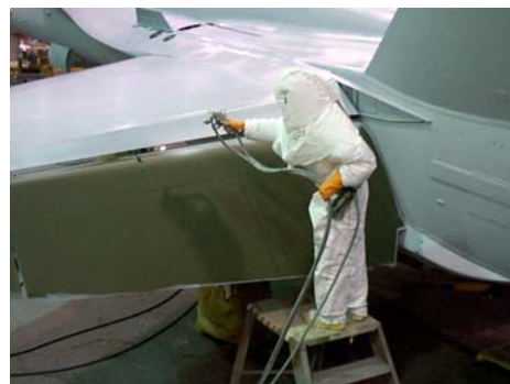
Figure 3. Zero-VOC Topcoat Application to Outer Wing Panel of C-2 (left) and F/A-18D at NADEP NORIS (right).
