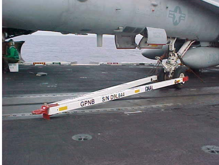
Figure 5. Tow Bars Painted with Zero-VOC Topcoat at NAVAIRSEFAC, Solomons, MD. Tow Bars are Deployed on USS Harry S Truman.
