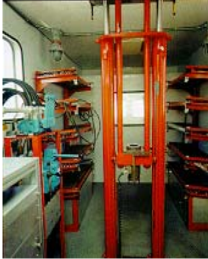
Figure 3. SCAPS Truck Hydraulic Rams.
