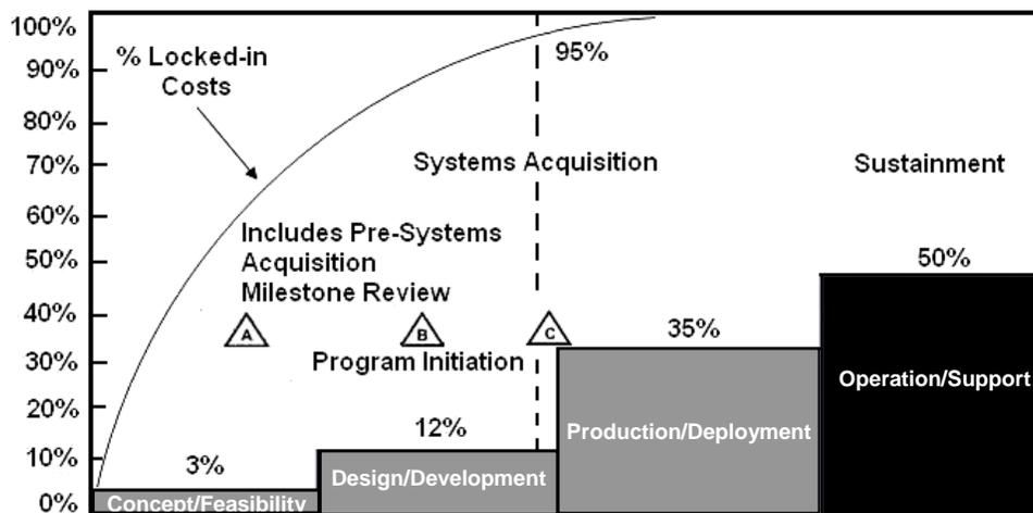
**Figure 4. PERCENT OF LIFECYCLE COSTS LOCKED-IN BY PHASES<sup>13</sup>**
